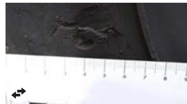
Banden: Nok > 3 mm diep, demontage
